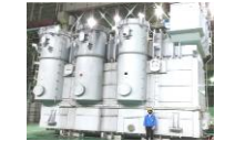
Large-capacity transformers (power transformation)
