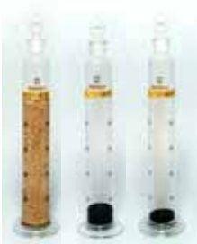
Performance of volume reduction (ion-exchange resin) (1/10-1/20)
