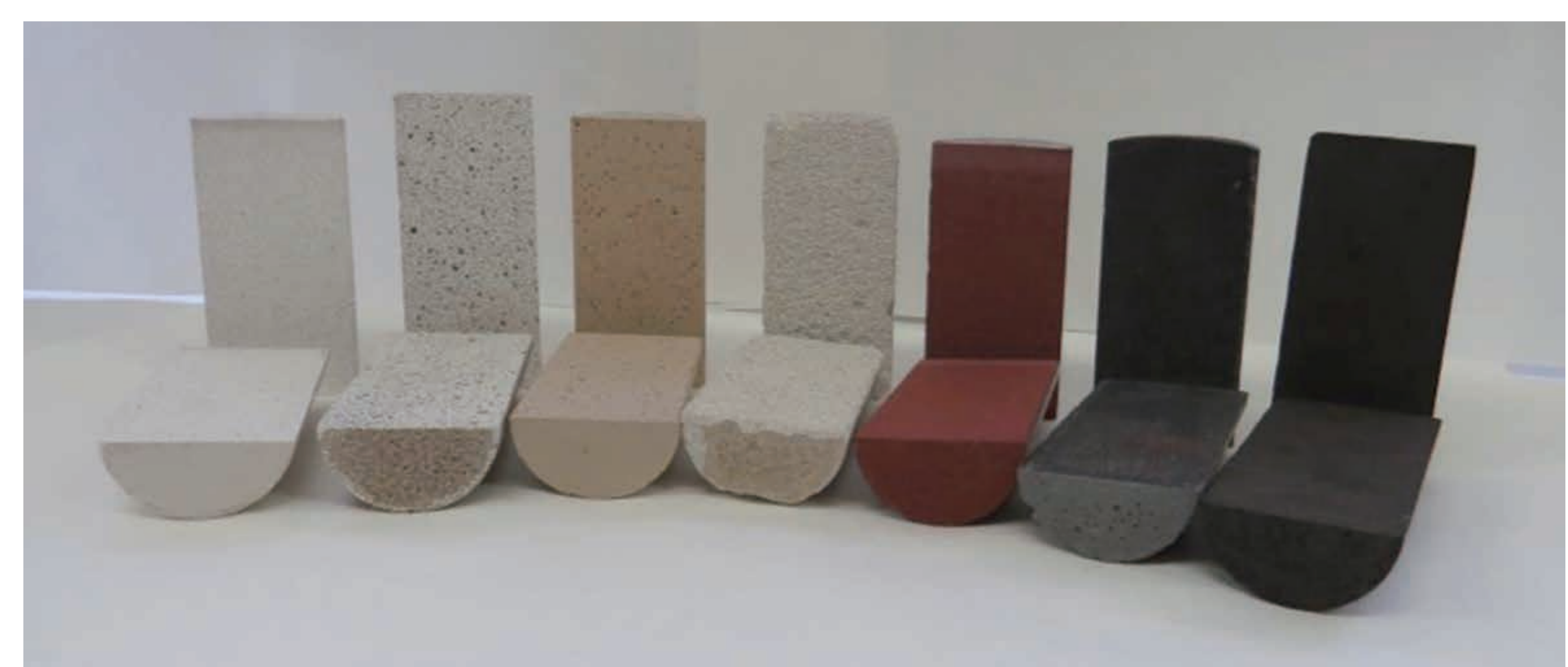
Figure 5: Samples solidified with SIAL® geopolymer
