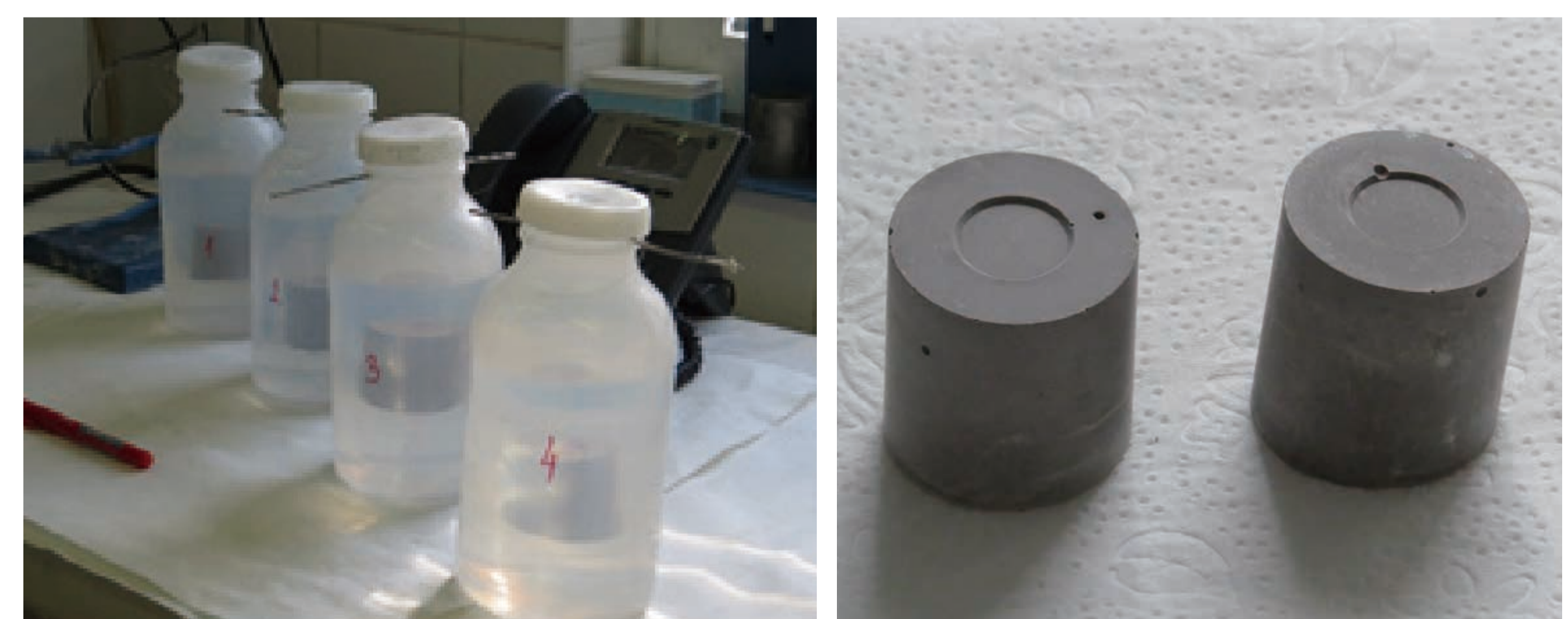
Figure 4: Samples of sodium sulphate solidification
