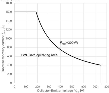
Notice)  $V_{CE}$  is defined between Sense P and Sense U/V/W for upper arm and Sense U/V/W and Sense N for lower arm.
