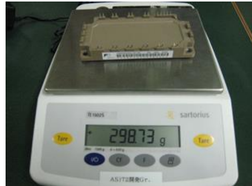
2. Measure weight of IGBT
